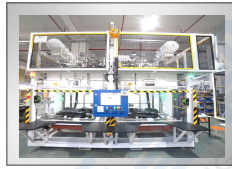
氦检漏 Helium leak detection
