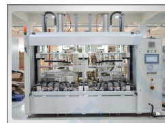
立柱焊接装备 Pillar welding machine
