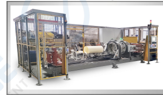
内胆瓶红外焊接切割 Infrared welding cutting machine for Internal gall bottle
