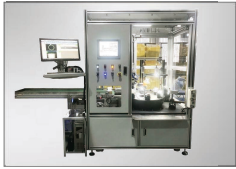
视觉外观、缺陷检测 Visual detection in appearance & defect
